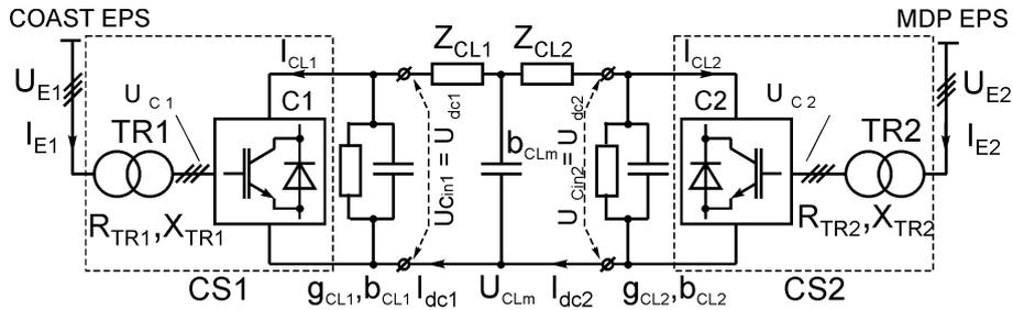
Fig.1. Equivalent circuit of HVDC light which concedes parasitic parameters of electrical equipment
