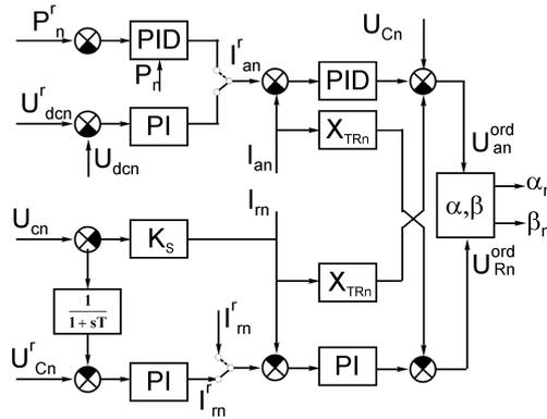
Fig.2. IGBT bridge converter control system
