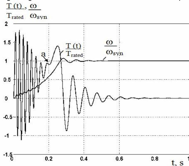
Fig.4. PC simulations of the no-loaded IM run up transient.
