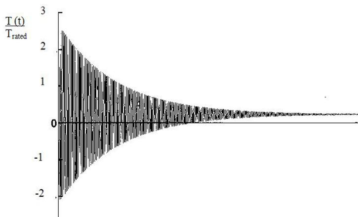
Fig. 1. A curve of transient torque in per units at direct switching on the standstill IM (series 4A180M4, P= 30 kW) to a grid.
