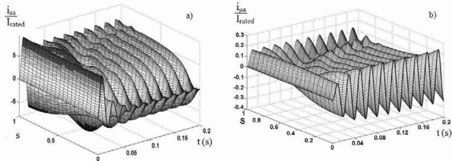
Fig. 2. Stator (a) and magnetizing (b) currents transient at direct switching on the rotating IM (series 4A180M4, P=30 kW) to a grid.
