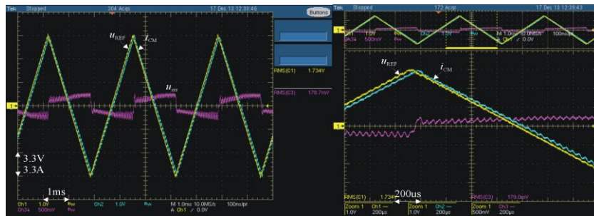
Fig. 15. Selected waveforms in the laboratory prototype of the current modulator: reference voltage, modulator current, and error signal while M=1 . The current modulator amplitude is equal to the nominal one.
