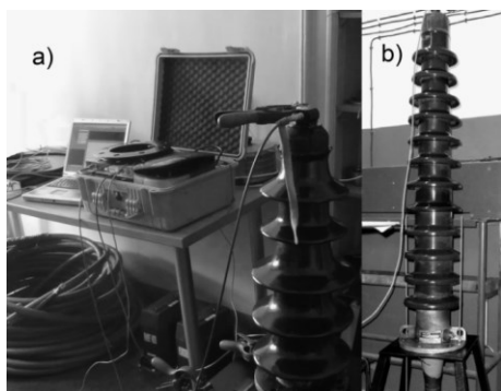
Fig.1. The research stand of the bushing CRTP (a) and the bushing CTFK (b).
